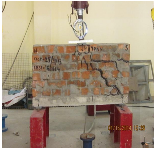
Figure 6.3.(a) Load-deflection curve ,(b) Lintel-Masonry Test Wall 4-Foot Span (6Layer Masonry) under concentrated loading.
