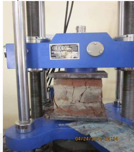
Fig. 5.3. Compression test of brick masonry blocks in UTM 40 tonne capacity.
