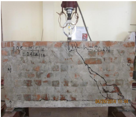
Figure 6.6.(a) Load-deflection curve ,(b) Lintel-Masonry Test Wall 6-Foot Span (8Layer Masonry) under concentrated loading.
