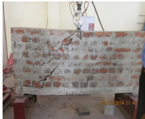
Figure 6.5.(a) Load-deflection curve ,(b) Lintel-Masonry Test Wall 6-Foot Span (8Layer Masonry) under concentrated loading.
