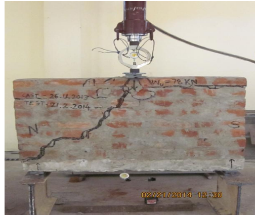
Figure 6.4.(a) Load-deflection curve ,(b) Lintel-Masonry Test Wall 4-Foot Span (8Layer Masonry) under concentrated loading.
