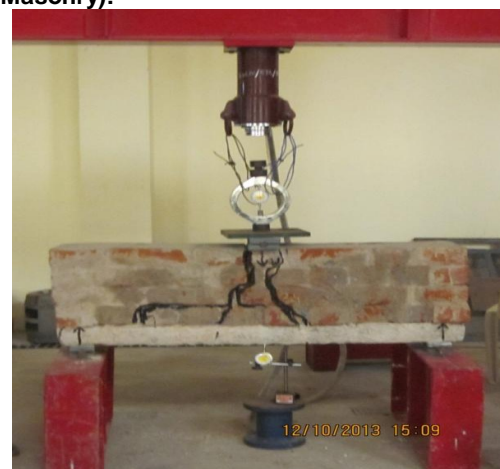
Figure 6.2.(a) Load-deflection curve ,(b) Lintel-Masonry Test Wall 4-Foot Span (4Layer Masonry) under concentrated loading
